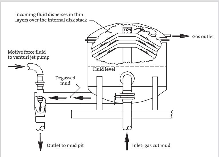
ensure that the disk stack is never submerged. As fluid level rises and lifts the float, air enters the vessel through the three-way valve to decrease the vacuum inside the vessel. With less vacuum inside the vessel, the rate at which fluid is drawn into the tank slows and the rate at which fluid exits the vessel increases. The fluid level inside the vessel drops rapidly until the
