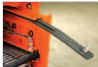
*Screen-clamping actuators designed with continuous toggle to allow installation from discharge end of shaker*
